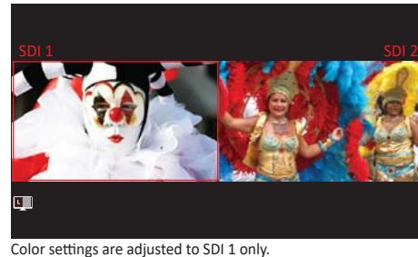
This unique function allows to display the same image side by side, change the color settings to one image, and then compare the original image and the changed image on the screen.
