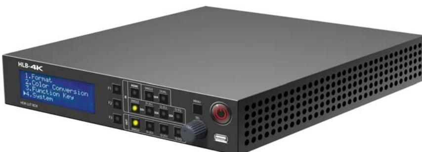
HLB-4K is a stand-alone converter which supports up-conversion and down-conversion between 4K and HD, HDR to SDR conversion and vice versa, color gamut conversion between BT.2020 and BT.709. And, the 12G-SDI single link video input can be output to 6G-SDI dual link or 3G-SDI quad link.
